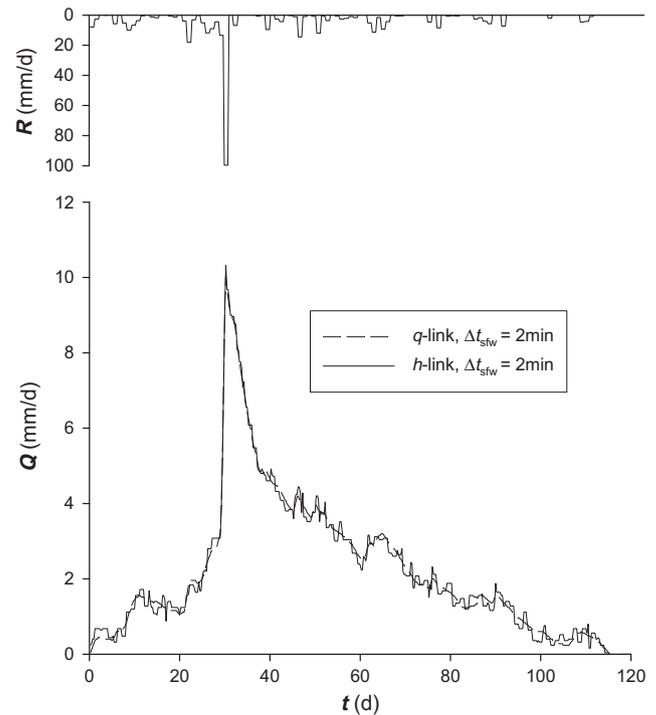
**Fig. 10.** Comparison between simulated peak flows (time averaged over 0.25 d) using the model of Fig. 9 with respectively an  $h$ -link and a  $q$ -link with a runoff resistance  $c$  of 0.083 d. The used surface water time step is 2 min. The recharge  $R$  of the model is here defined in terms of the total precipitation minus the total actual evapotranspiration.
