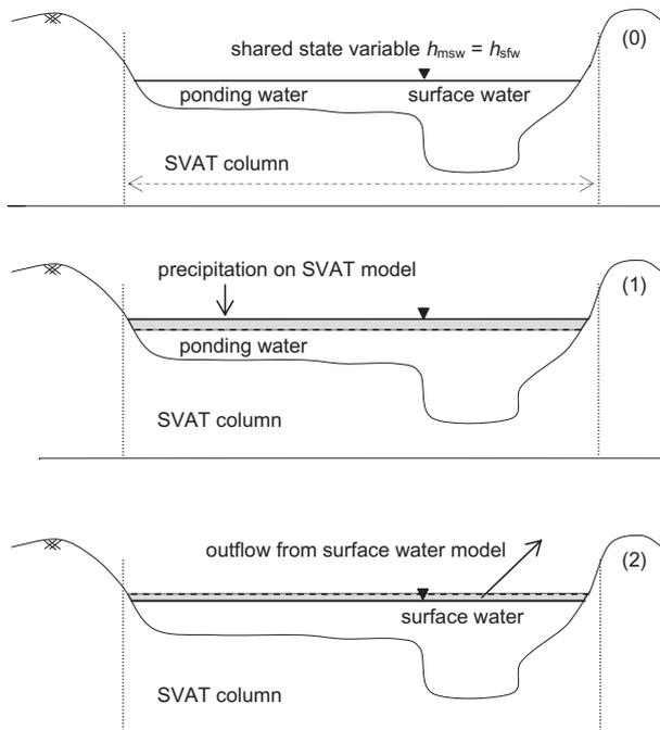
**Fig. 5.** Computational steps of integrated model for ponding water ( $h_{msw}$ ) and surface water ( $h_{sfw}$ ).
