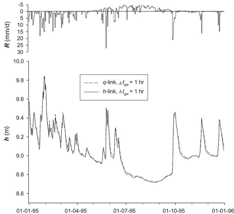
Fig. 7. Comparison between simulation results for the phreatic level  $h$ , using the  $q$ -link and the  $h$ -link coupling method, for the location in the test model indicated in Fig. 6. The plotting time interval is 1 d. The recharge  $R$  has been taken as the infiltration at the soil surface minus the actual transpiration.
