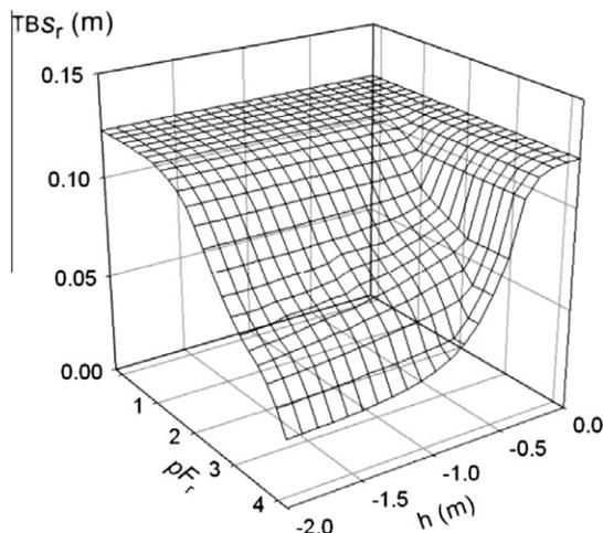
Fig. 2. Example of a bivariate tabular root zone storage function  $\mathbf{tbs}_r(\psi_r, h)$  for a loamy soil with a root zone thickness of 0.30 m. The total storage in the root zone is a function of the mean pressure head in the root zone (pF of  $\psi_r$ ) and the phreatic level ( $h$ ).
