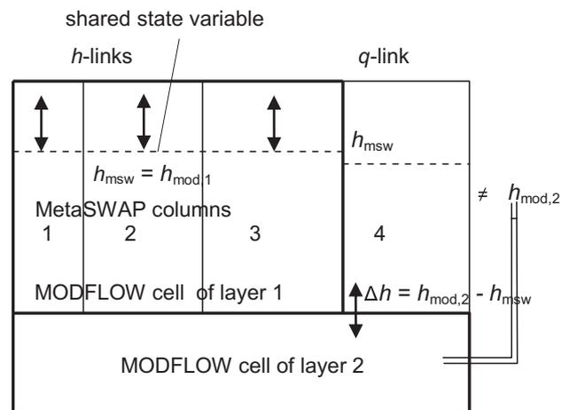
Fig. 1. Cross-section of the MetaSWAP-MODFLOW coupled systems, showing examples of so-called *h*-links via a shared state variable (phreatic level  $h_{msw}$ ) on the left, and a flux link ('*q*-link') on the right.
